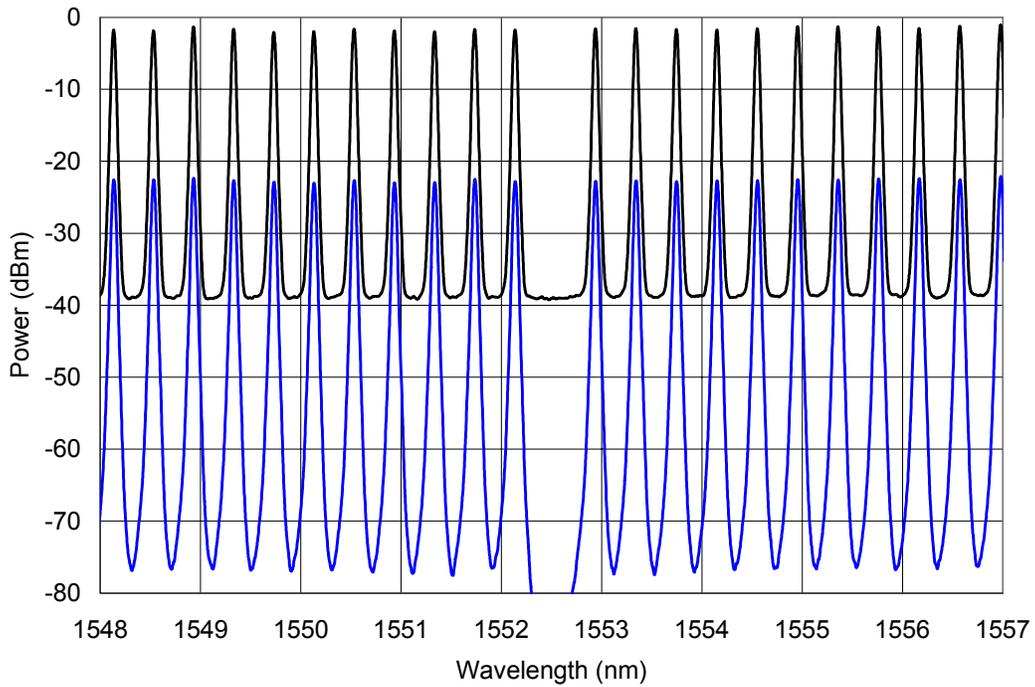
Fig.3. Comb spectra at the input and output of the EDFA measured with an OSA resolution of 0.02 nm.
