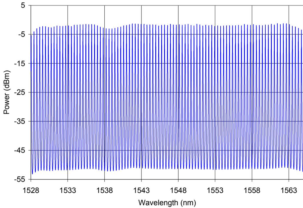
Fig.1. Emission spectrum of the ASE-sliced 50-GHz spaced comb source.
