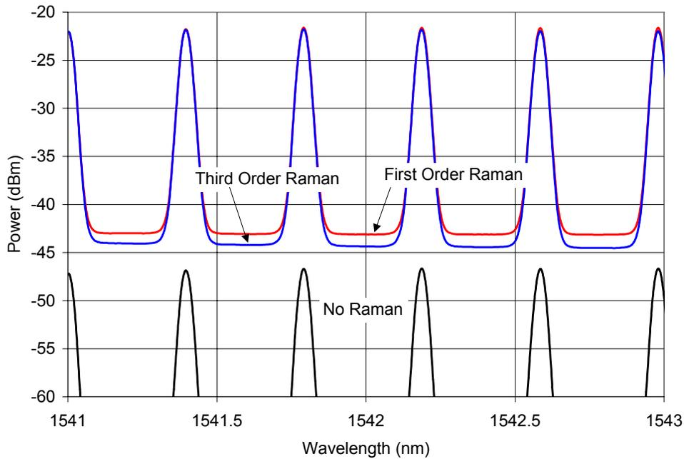
Fig.7. Comb signal spectra measured at the link output when the Raman pump was turned off, and amplified signal when the link was pumped by first- and third-order Raman pumps.
