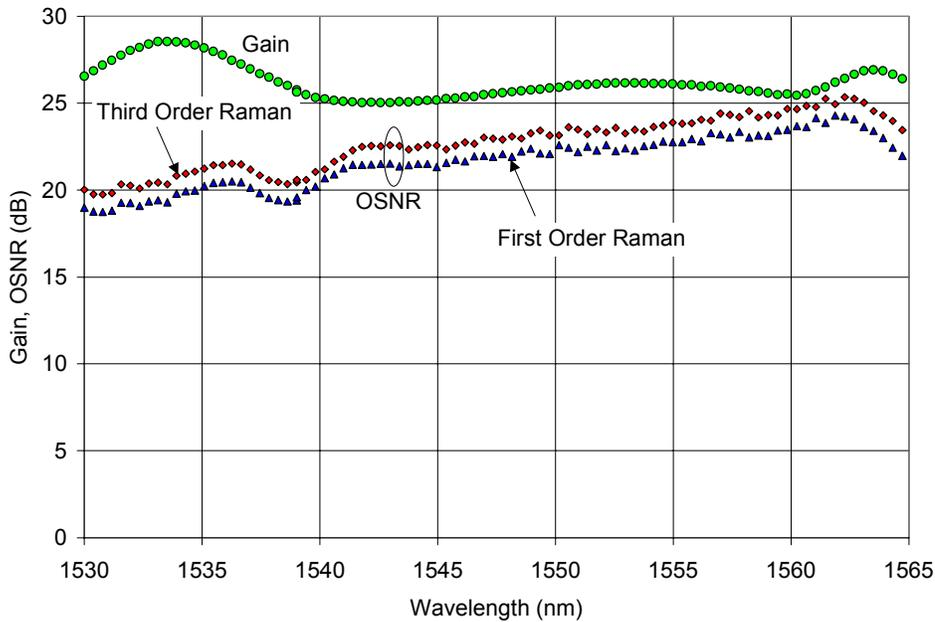
Fig.8. On/off Raman gain spectra and OSNR measured at the output of the link when pumped by the first- and third-order dual-wavelength Raman pumps.
