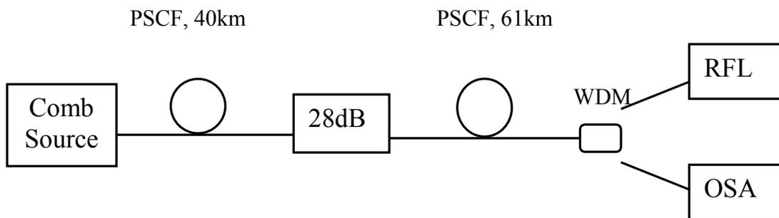
Fig.5. Experimental set-up for testing 255-km PSCF link with Raman amplification.
