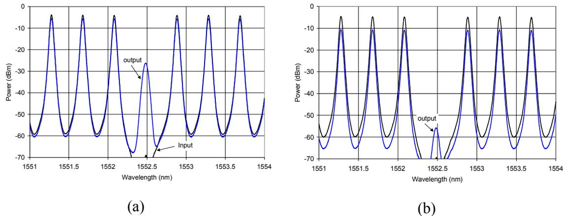
Fig.9. Central part of the comb spectra measured at after 6 km of dispersion shifted fiber (a) and 23 km of TrueWave fiber (b). Composite input signal power in both cases was 18 dBm.
