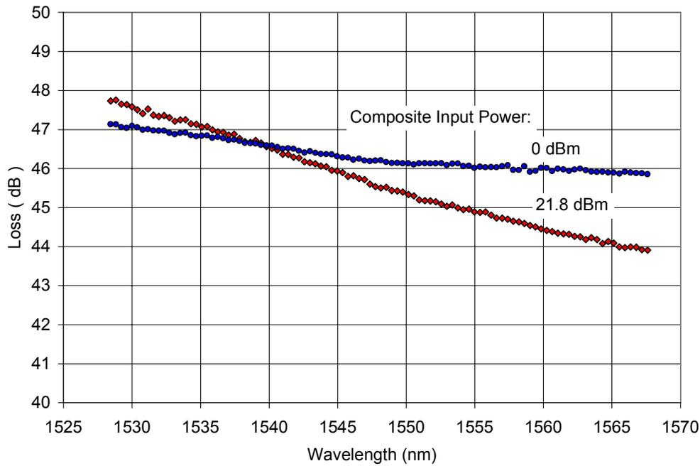
Fig.6. Attenuation of the DWDM signal in a PSCF link measured at two different composite powers.
