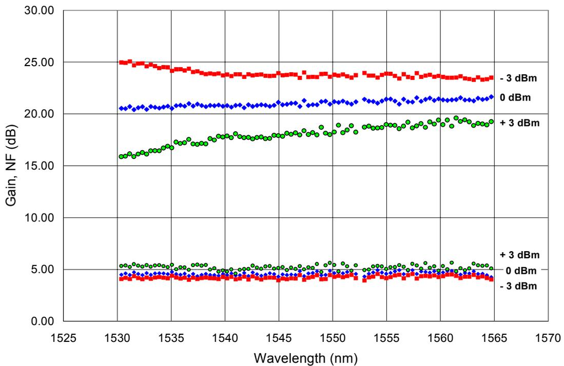
Fig.4. Gain and Noise Figure of EDFA measured at composite input powers of -3, 0 and +3 dBm.
