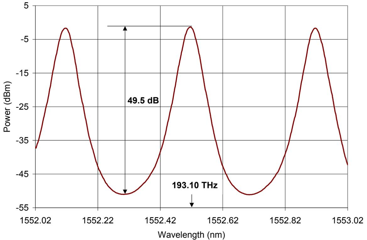
Fig.2. Emission peaks are anchored to ITU grid.
