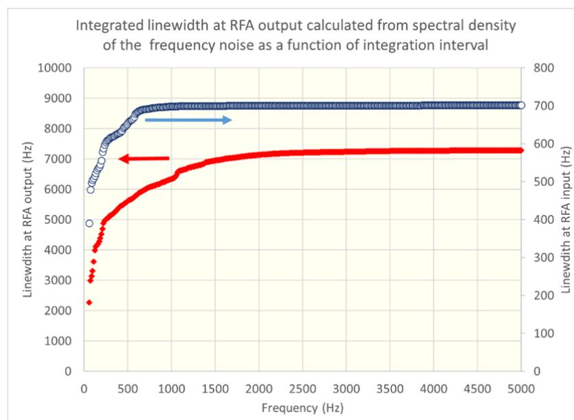
Fig. 11 Integrated spectral linewidth of the seed before and after amplification.
