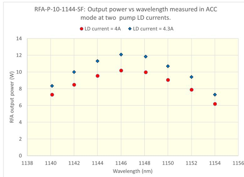
Fig. 6. RFA output power as function of the seed laser wavelength. Seed power 11 mW.
