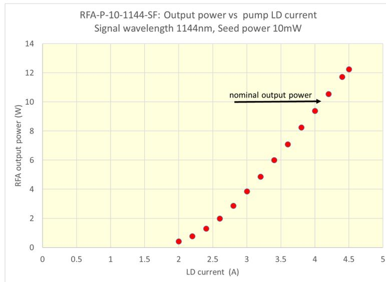
Fig. 3. Output power of 1144-nm RFA as function of pump LD current.
