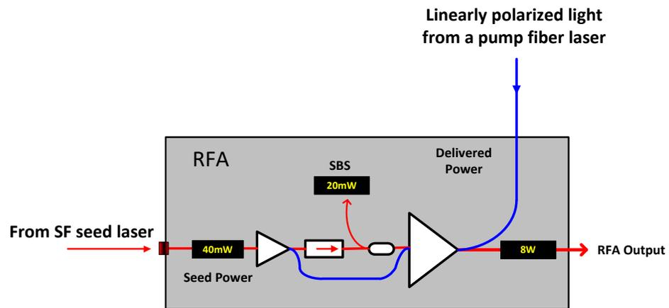
Fig. 1. Diagram of Raman Fiber Amplifier (RFA-SF series).
