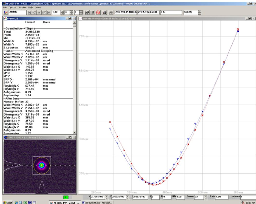
Fig. 13. Beam evolution along propagation axis taken at the output 4-W 628nm VRFA reveals  $M^2$  of 1.05 and 1.02 in X and Y axii.
