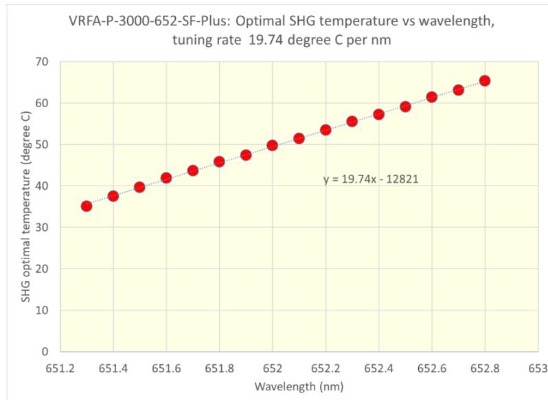
Fig. 7. SHG crystal optimal temperature as function of the seed wavelength measured in VRFA-P-3000-652-SF.
