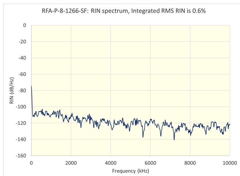
Fig. 8 RIN spectrum measured at the output of 8-W 1266-nm RFA. Integrated across 10MHz RMS RIN is in the order of 0.6%.
