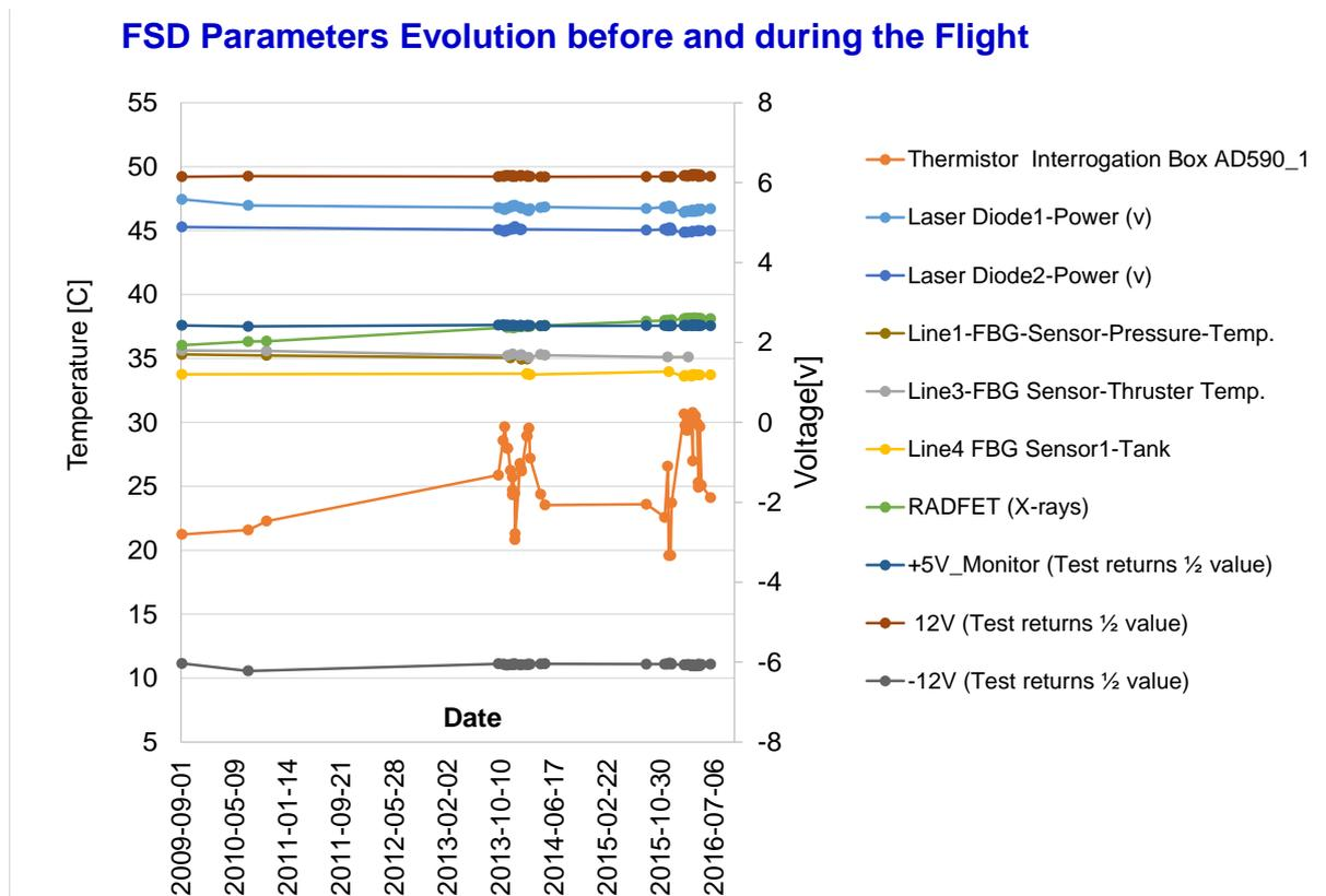
Fig. 8: Main FSD parameter evolution since the last on ground measurement. Only the temperature follows the primary vertical axis (left side), all the other parameters follows the secondary axis (right)
