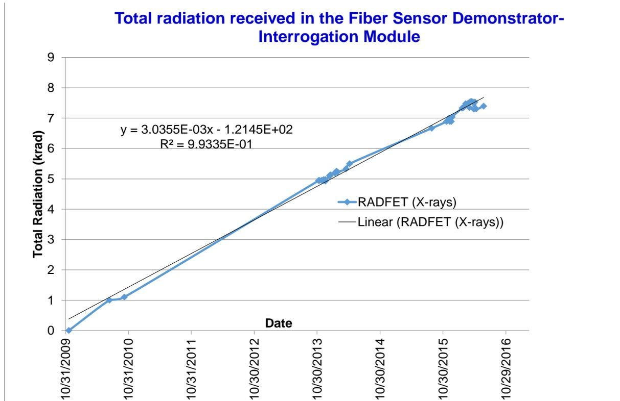
Fig. 9: Calibration of the RADFET vs the time spent in space
