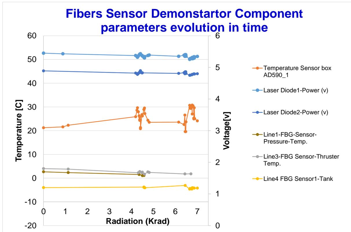
Fig. 10: Main FSD parameter evolution since the last on ground measurement
