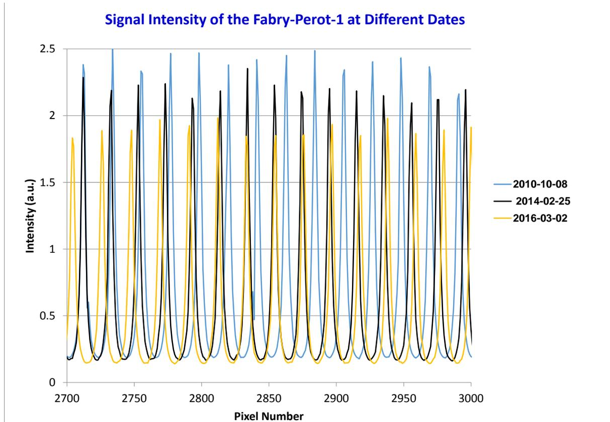
Fig. 7: Intensity of the fixed Fabry Perot Scans (50 GHz/scan) in a Zoom over the pixels 2700-3000 of the tuneable Fabry-Perot (total 45 nm/ 4000 pixel width)
