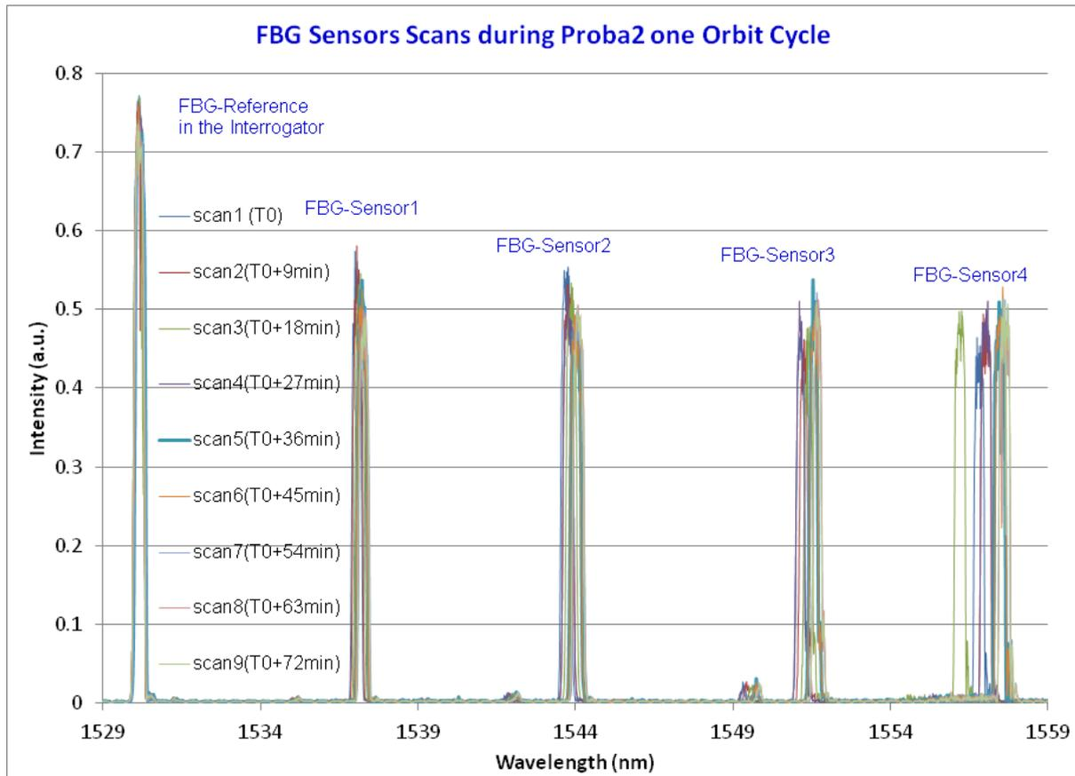
Fig. 5: Scan of the wavelengths of the Line during the orbit cycle
