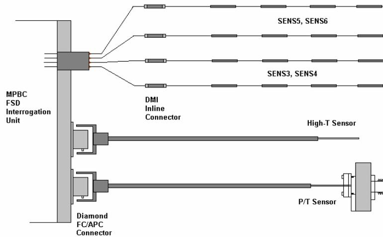
**Fig.1 Schematic of FSD fiber-optic sensor signal harness.**
