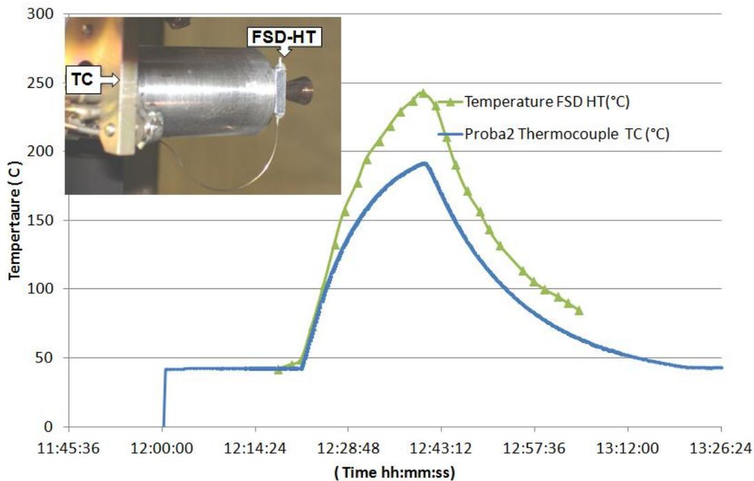
**Fig. 4: Temperature measurements with FBG sensor at the thruster top, and a thermocouple at the thruster bottom, during a preheat experiment**
