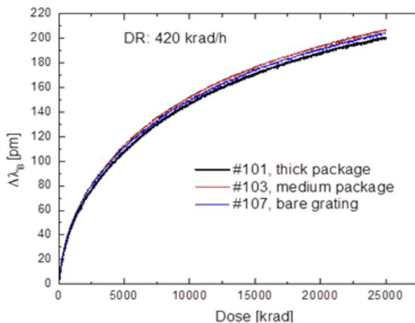
**Fig. 11: Central-Wave-Length shift with 25 Mrad at a dose rate of 420rad/h**
