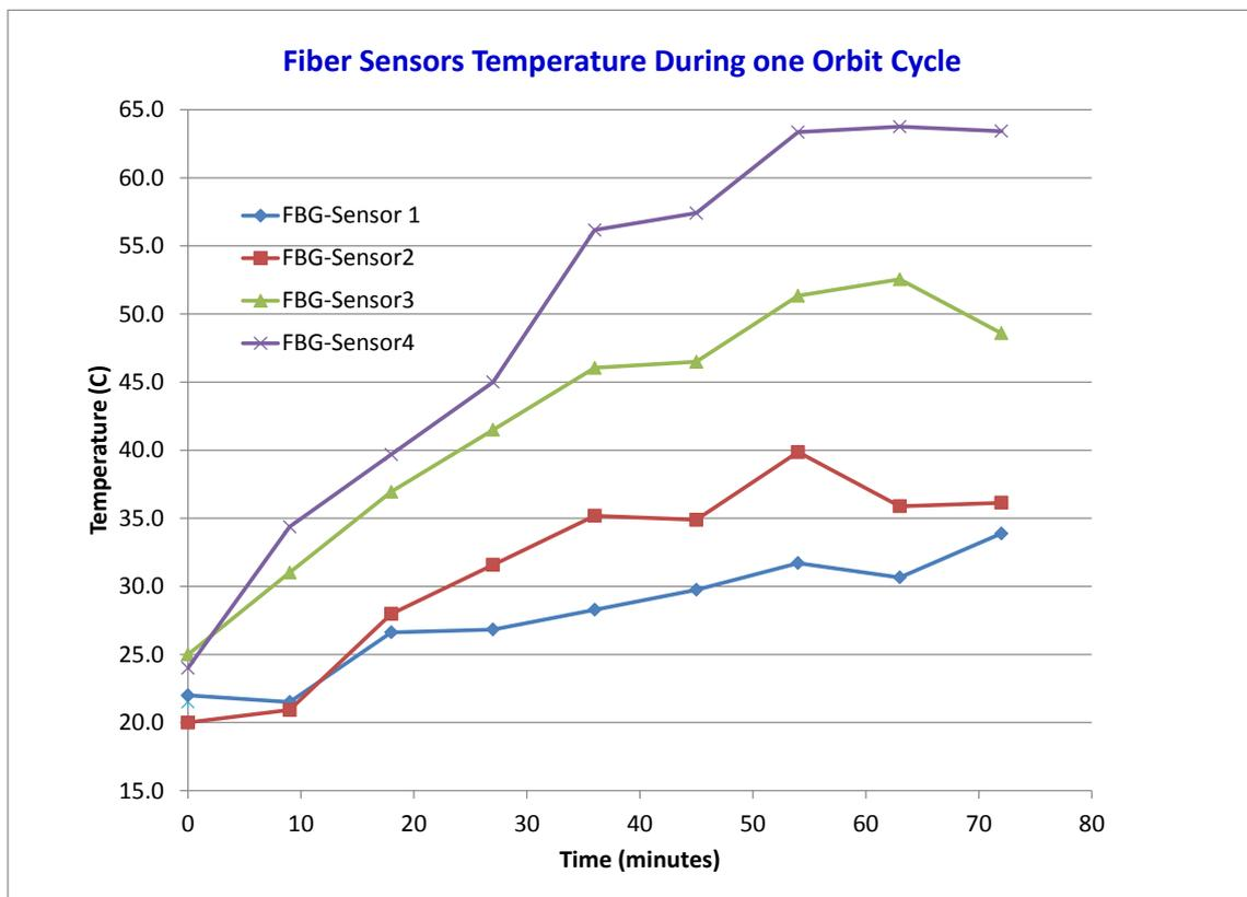
Fig. 6: Temperature measurements provided by the four sensors of Fiber Line\_sens6(Bus)
