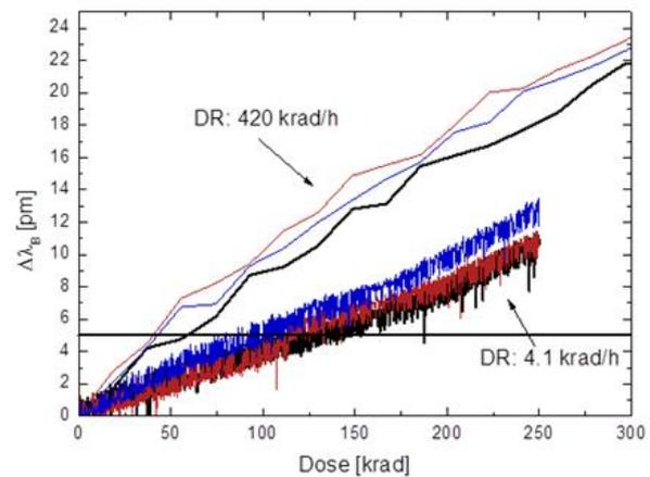
**Fig. 12: CWL shift at 300 krad total dose, comparison of two dose rates ( 420 vs 4.1 rad/h)**
