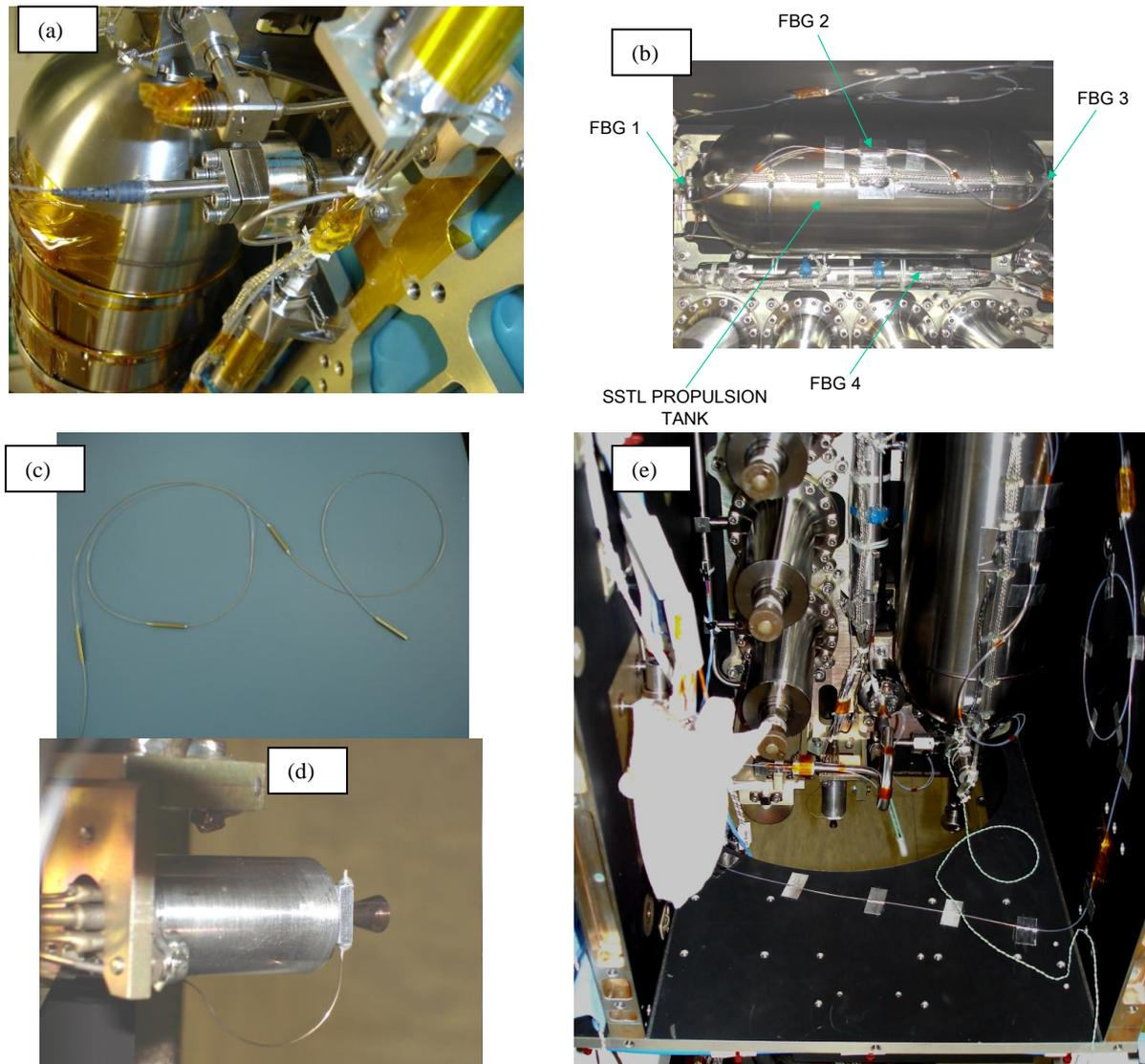
**Fig. 2: Photograph of flight P/T sensor integrated with the SSTL propulsion system for Proba-2**
