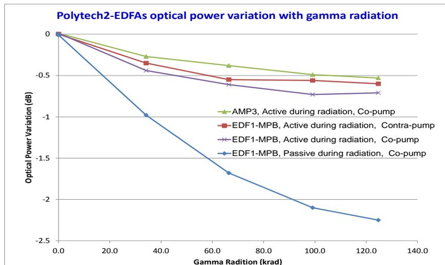
Fig. 5: Polytech-2 Gain Losses from the total power measurements
