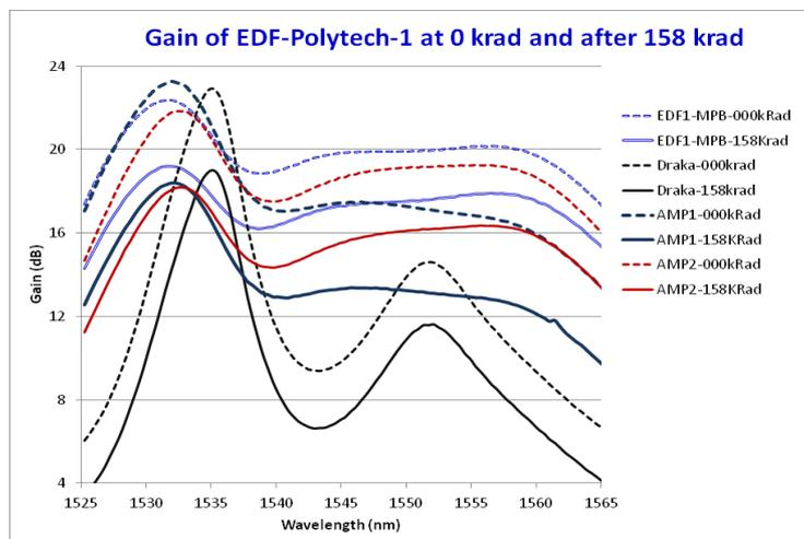
Fig. 4: Polytech-1 Gain spectra before (dashed lines) and after 158 krad the shape is kept
