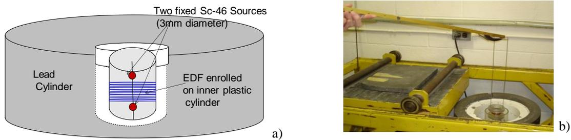
Figure 1: set up at Ecole Polytechnique Montreal using Sc-46- a) schematic and b) picture
