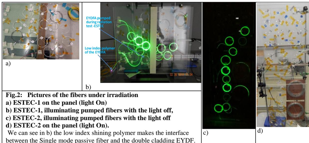
Fig.2: Pictures of the fibers under irradiation
