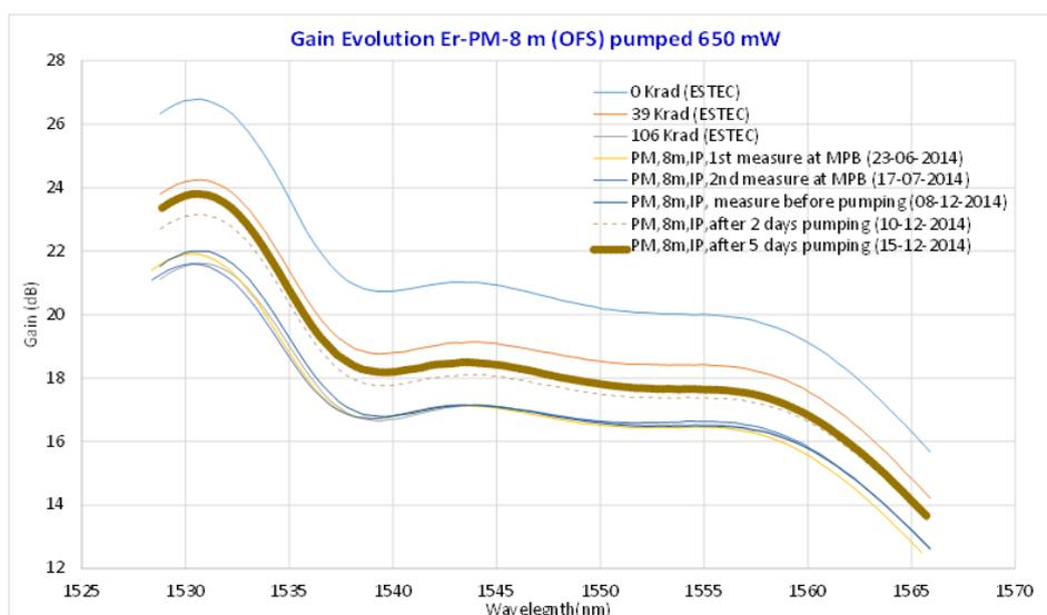
Fig. 8: Evolution of EDF-PM from OFS, Irradiated, pumped during irradiation at 650 mW
