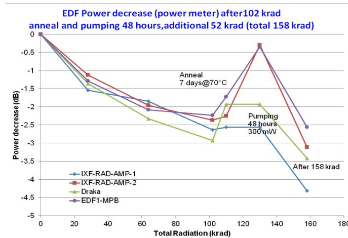
Fig. 3: Polytech-1 Total optical power evolution of the four fibers during the radiation from 0 to 102 krad, followed by an annealing of one week at 70°C, then 48 hours pumping (300 mW at 976 nm) and additional 56 Krad up to 158 krad.
