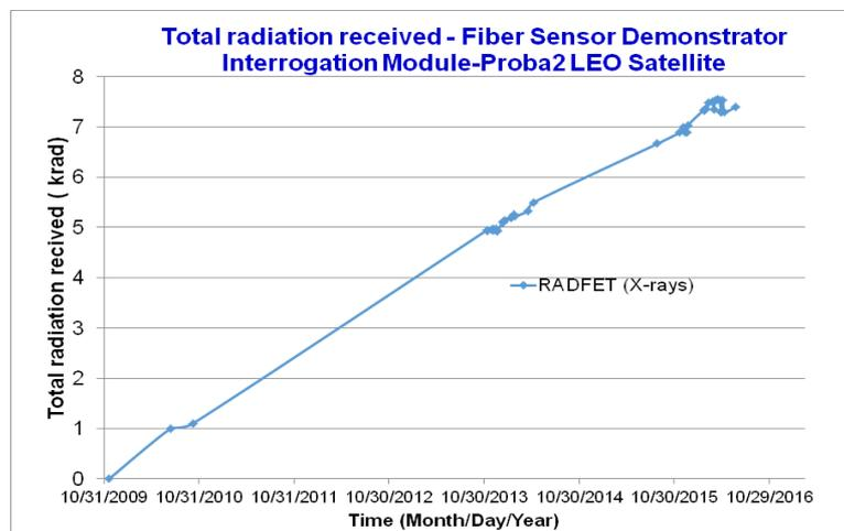
Fig. 9: Total Radiation received in the FSD- during the 7 years flight.
