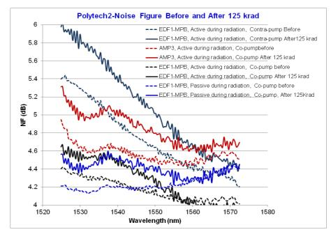
Fig. 6: Polytech-2 Noise Figure before (dashed lines) and after 125 krad
