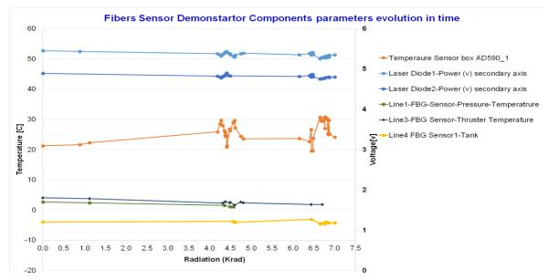
Fig. 10: Evolution of different components as function of the radiation from the Fig.9
