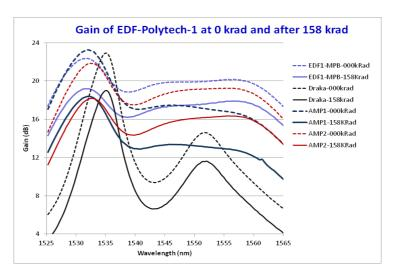
Fig. 4: Polytech-1 Gain spectra before (dashed lines) and after 158 krad the shape is kept
