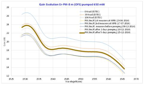
Fig. 8: Evolution of EDF-PM from OFS, Irradiated, pumped during irradiation at 650 mW
