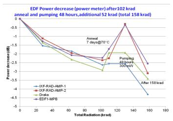
Fig. 3: Polytech-1 Total optical power evolution of the four fibers during the radiation from 0 to 102 krad, followed by an annealing of one week at 70°C, then 48 hours pumping (300 mW at 976 nm) and additional 56 Krad up to 158 krad.
